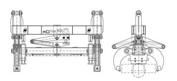
Heppenstall billet tongs are designed to accommodate custom billets of all dimensions with or without rotating unit.
