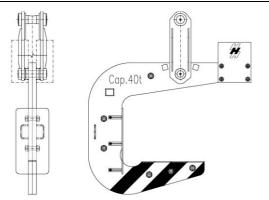
Heppenstall C-Hooks are designed to accommodate custom coils of all dimensions with or without rotating unit.
